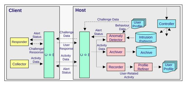
**Figure 3 : The Intrusion Monitoring System architecture**
