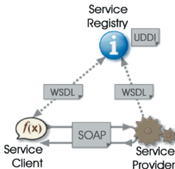
Figure 2. SOAP, WSDL and UDDI interaction scheme.
