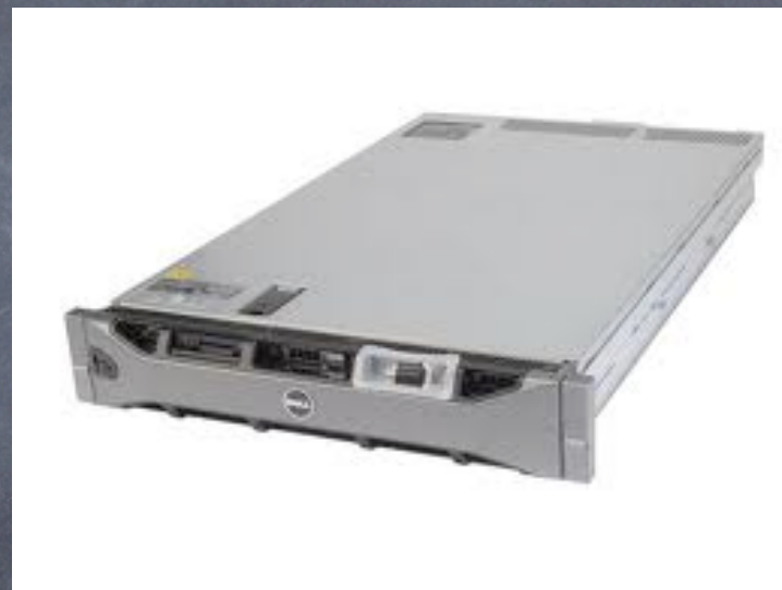
Dell R815 Memory fat node - 32 cores- 512 Gbytes of RAM
